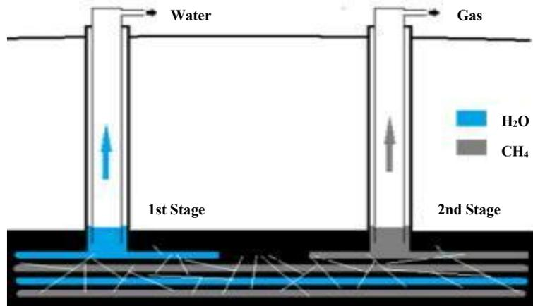
Figure 3—Vertical well showing stages of CBM production.
