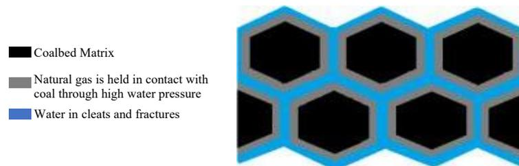
**Figure 1—Coalbed matrix illustrating gas surrounding the coal bounded by water and rock.**
