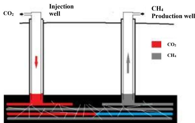
**Figure 7—Vertical well showing  $\text{CO}_2$ -ECBM recovery.**
